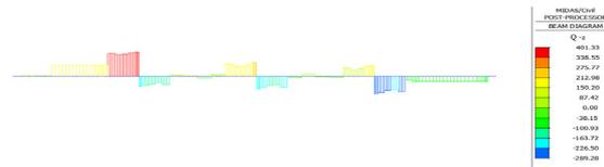
Figure 11 Shear diagram of the main cross-beam 1600 x 2700 mm under systematic heating-up condition
