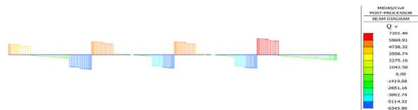
Figure 4 Shear diagram of the main cross-beam 1600 x 2700 mm under dead load
