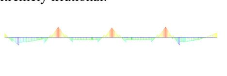
Figure 3 Bending moment diagram of the main cross-beam 1600 x 2700 mm under dead load
