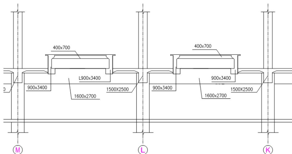
Figure 1 Vertical section of the rail layer for Harbinxi Railway Station layout
