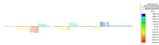
Figure 13 Shear diagram of the main cross-beam 1600 x 2700 mm under systematic cooling condition
