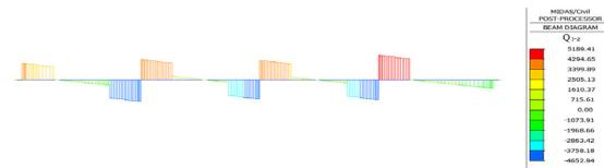
Figure 9 Shear diagram of the main cross-beam 1600 x 2700 mm under dead load under dead load
