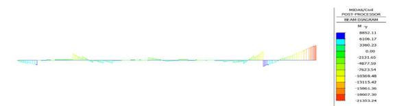
Figure 6 Bending moment diagram of the main cross-beam 1600 x 2700 mm under systematic cooling
