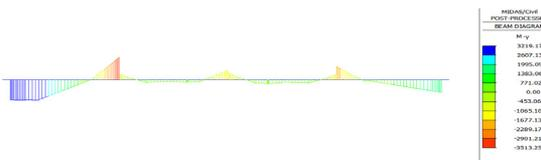
Figure 12 Bending moment diagram of the main cross-beam 1600 x 2700 mm under systematic cooling condition
