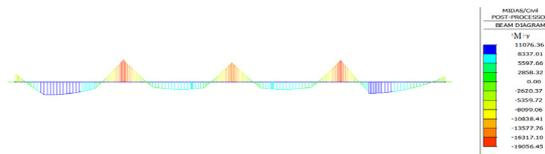
Figure 8 Bending moment diagram of the main cross-beam 1600 x 2700 mm
