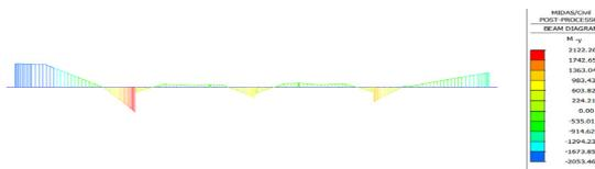
Figure 10 Bending moment diagram of the main cross-beam 1600 x 2700 mm under systematic heating-up
