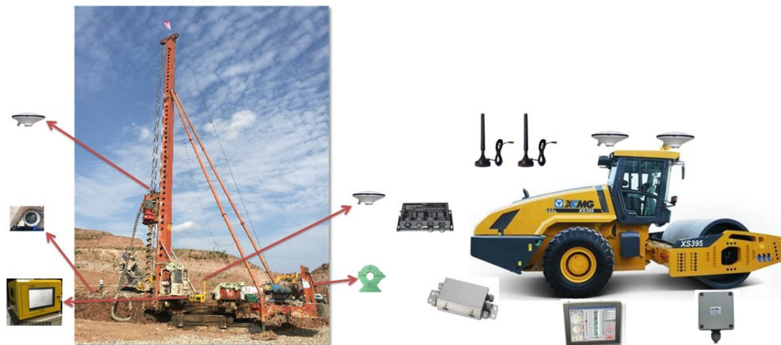
Figure 1. Digital construction system for construction machine in airport (left: CFG pile system; right: Vibration Roller system).
