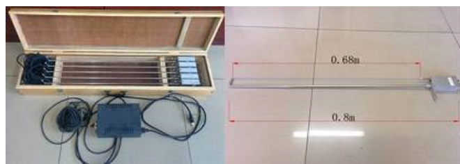
Figure 6 Waveform meter for waveform calibration
