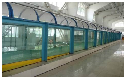
Figure 5 Wave flume for the model test
