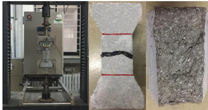
Figure 1. Loading device for the uniaxial tensile test and failure modes of SPHFC under uniaxial tension
