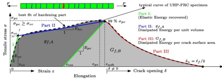
Figure 3. Stress-strain and Idealized Modeling Method of Typical Ultra-high Performance Fiber Reinforced Concrete [6]
