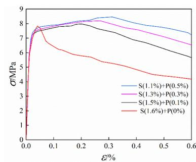
Figure 6. Simulated stress-strain curves of different fiber combinations under uniaxial tension
