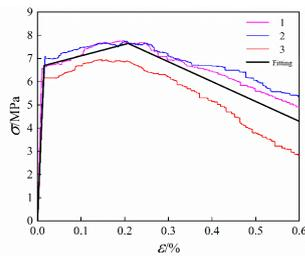
Figure 2. Stress-strain curves of SPHFC 120 under uniaxial tension and fitting curve
