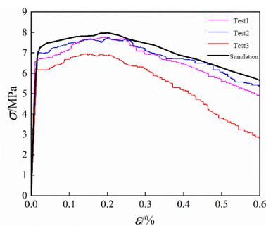
Figure 5. Comparison between test and Simulation of stress-strain curves of SPHFC120 under uniaxial tension
