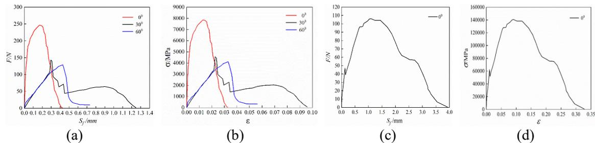
Figure 4. Constitutive relation of steel fiber and PVA fiber<sup>[9,10]</sup>: (a) Load slip curves of steel fiber; (b) Stress-strain curves of steel fiber; (c) Load slip curve of PVA fiber; (d) Stress-strain curve of PVA fiber
