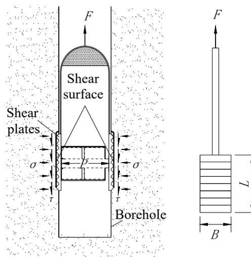
Figure 3. Schematic of borehole shear test principle.
