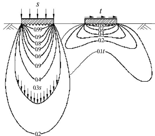
Figure 4. Normal and shearing stress distribution in elastic medium.
