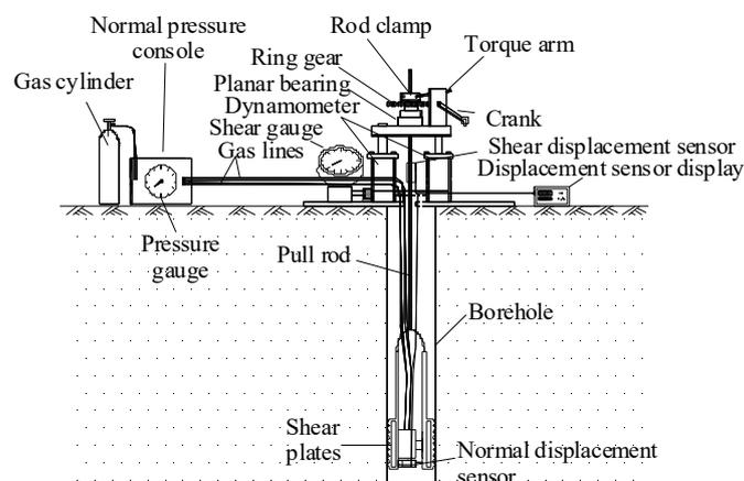
Figure 2. Schematic of improved borehole shear test device.
