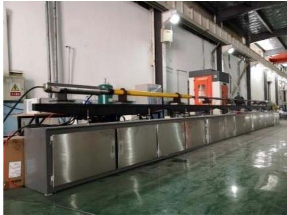
**Figure 1.** Photo of the SHPB impact system
