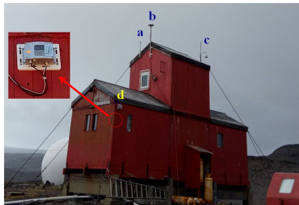
Figure 2. Meteorological station at Carlini Base, Antarctica for (a) LD-350 lightning Sensor, GPS antenna, (c) Electric Field Mill (EFM-100) antenna, and (d) Vaisala PTU300 sensors.
