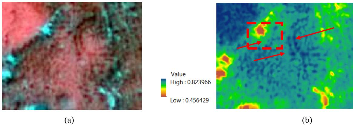
**Figure 3.** (a) The image (subset) of the study area after through image filtering using the Erdas Image 2020 software. (b) The classification image in each color defined the classes' areas. A red dotted square shows where the location of resistivity measurement has been done (Department of Geology, USM, 2017). It is predicted that the shape of the curve (see arrows) is a small stream or river based on the elevation profile in Figure 1.
