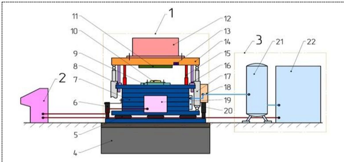
**Figure 4.** Structure of shock machine SMU1200: 1 – shock machine; 2 – control stand; 3 – compressor; 4 – foundation; 5 – balloon pneumatic cylinder; 6 – shock absorber; 7 – inertial block; 8 – sliding sleeve; 9 – anvil; 10 – shaping device; 11 – open die; 12 – test object; 13 – shock accelerometer; 14 – shock table; 15 – parking racks; 16 – table guide; 17 – pneumatic actuator; 18 – pneumatic drive equipment; 19 – switching unit; 20 – pneumatic unit; 21 – receiver; 22 – compressor
