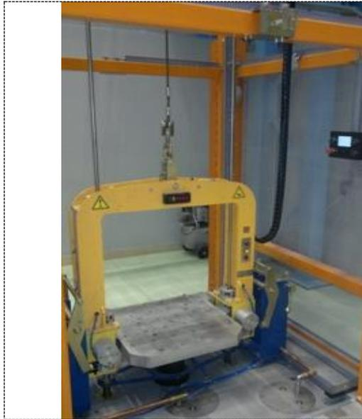
**Figure 2.** Dropper and shock table
