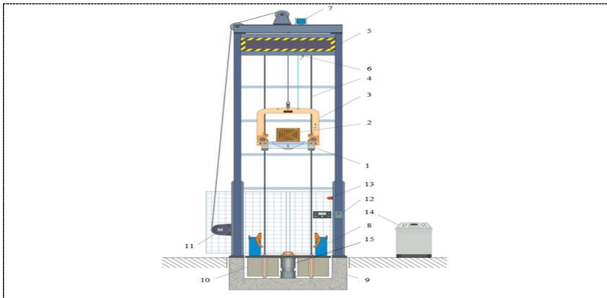
**Figure 1.** Scheme of shock machine KSP5: 1 – shock table; 2 – test object; 3 – dropper; 4 – guides; 5 – shaft; 6 – emergency limit switch; 7 – lift height sensor; 8 – parking device; 9 – foundation; 10 – inertial block; 11 – winch; 12 – auxiliary control panel of the machine; 13 – flashing beacon; 14 – operation panel; 15 – pneumatic cylinder of the sleeve type
