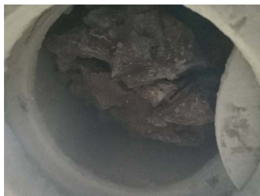
Figure 1. Blocked short pipe for ash discharge.
