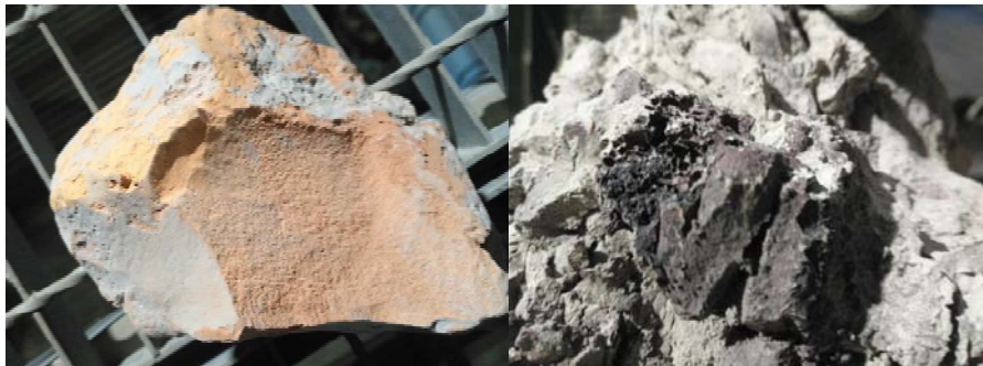
Figure 2. Appearance inspection of coke.
