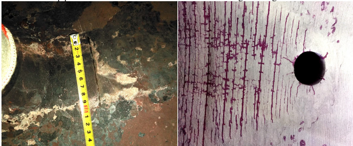
Figure 2 Cracks on the outer wall of the pipeline Figure 3 Cracks in the inner wall of pipeline
