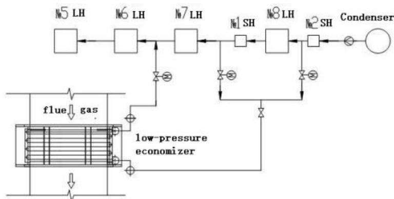
Figure 2. Schematic diagram of low-pressure economizer
