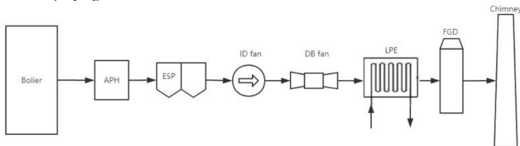
Figure 1. Schematic diagram of installation position of low-pressure economizer
