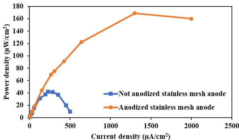
**Figure 5.** The power density of the batteries using the anodes with and without anodization.
