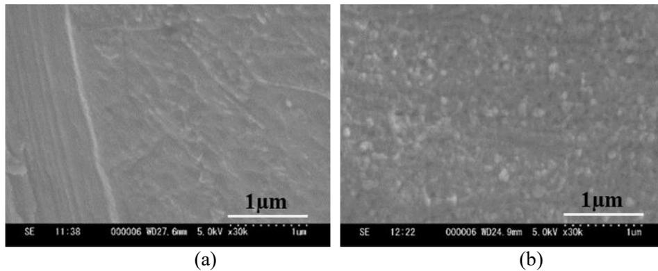
**Figure 4.** SEM images of the stainless mesh without anodization (a) and the anodized stainless mesh (b).
