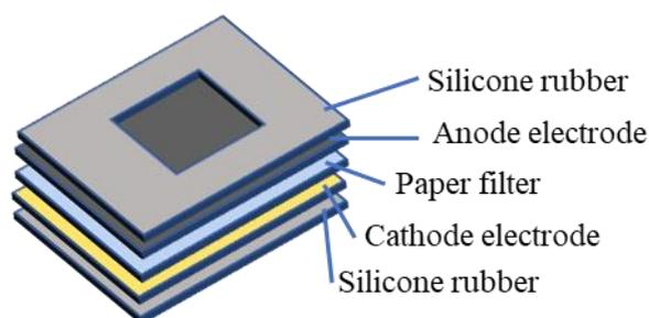
**Figure 2.** Structure diagram of the battery.
