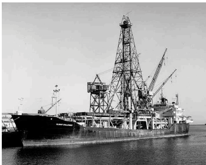
Figure 1. Special drilling vessel «Glomar Challenger».
