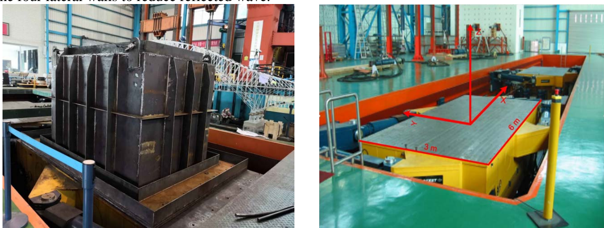
Figures 2. The tank on shaking table (left) and the details of shaking table (right).
