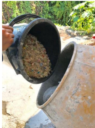
Figure 2. The making of PET concrete block.
