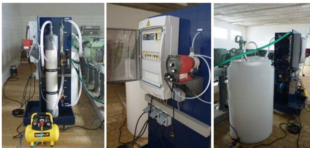
Figure 3. A view of the ultrafiltration device, the membrane module itself, the control system and the treated water storage tank.
