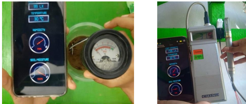
Figure 7. Measurement between Virtuino app and standard instrument
