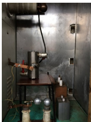
Figure 2. The actual model of the device for electro-hydraulic treatment of solutions
