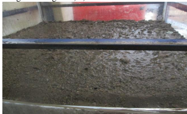
Figure 1. Model of embankment in rainfall simulator tool. Length 100 cm, Width 120 cm, height 40 cm
