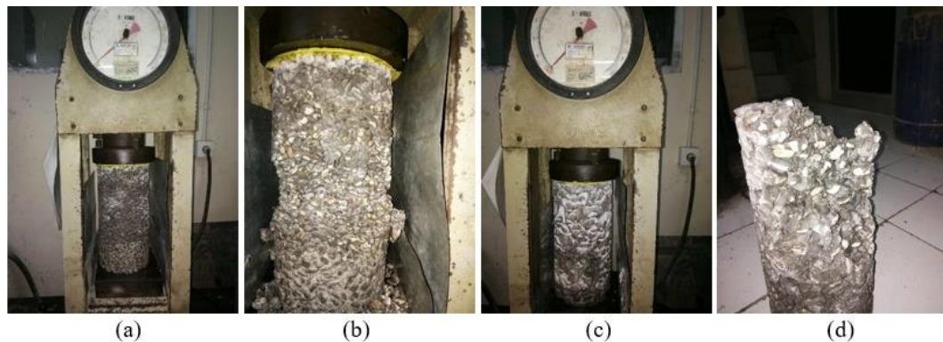
Figure 8. Compression strength test (a) sample with (9.5 - 4.75) mm natural aggregate, (b) typical collapse after compression for (9.5 - 4.75) mm natural aggregate, (c) sample with (19.0 - 12.5) mm (d) typical collapse.
