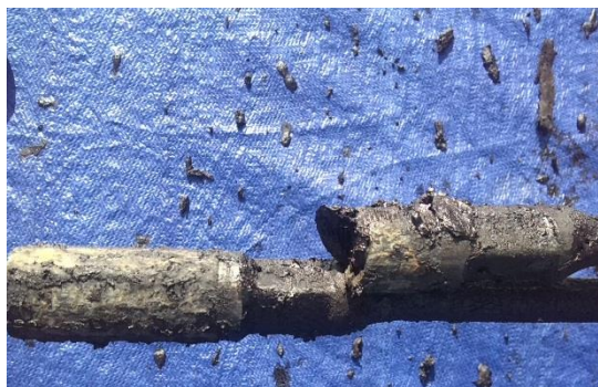
Figure 1. The wells of rod broken.
