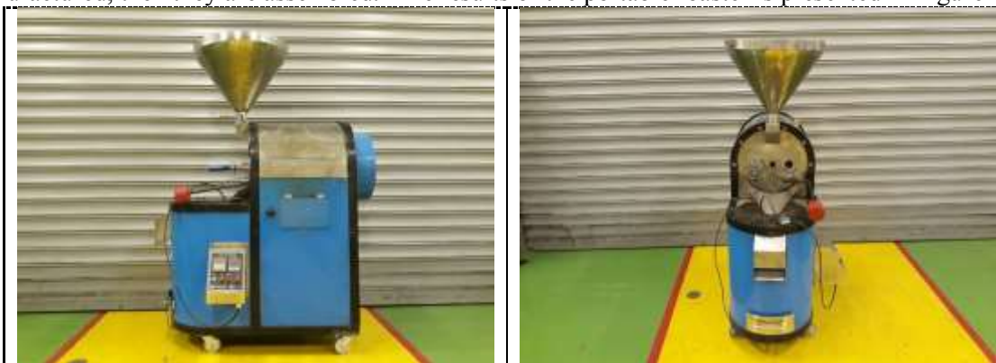
Figure 2. Portable coffee roaster machine for home industry scale
