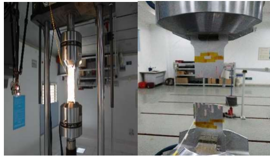
Figure 4. Comparison of fatigue testing machine before and after stretching
