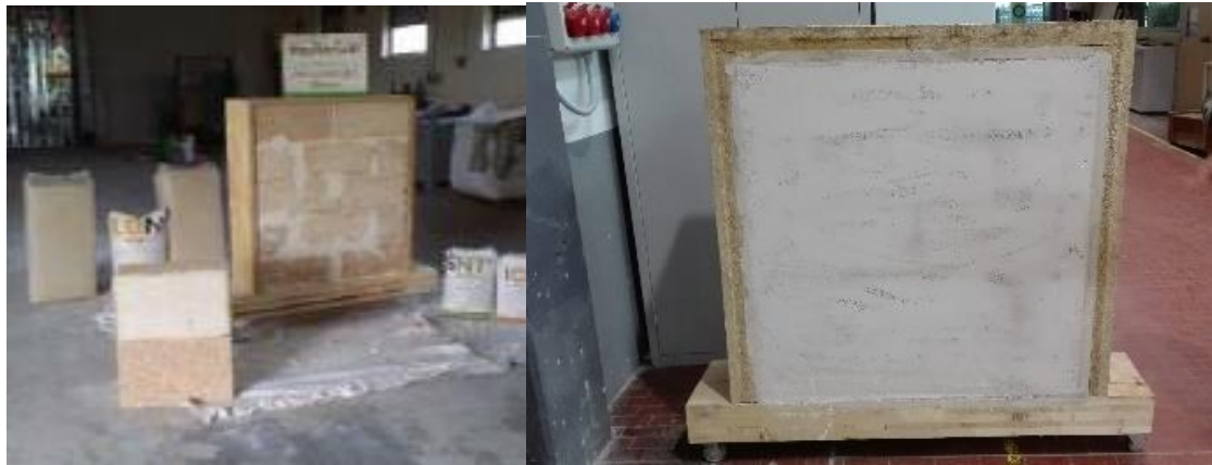
Figure 4. Hempcrete blocks' wall in the framework
