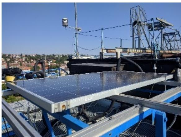
**Figure 2.** Unglazed PVT collector with sheet and tube absorber (VAR1)
