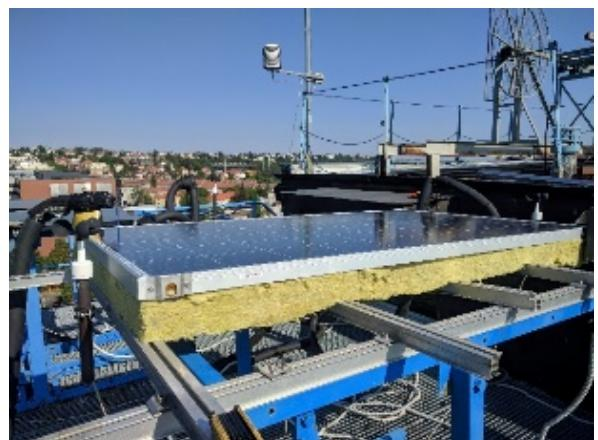
**Figure 3.** Unglazed PVT collector with sheet and tube absorber – insulated on the back side (IVAR1)
