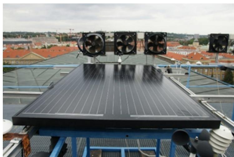
**Figure 4.** Unglazed PVT collector with polymer absorber (VAR2)
