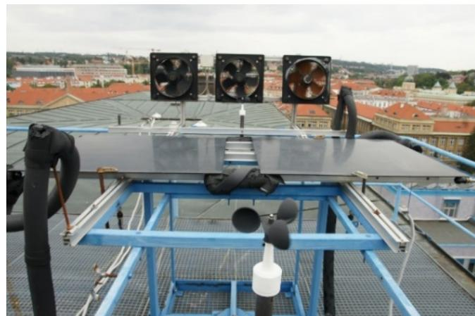
**Figure 1.** Reference unglazed solar thermal collector
