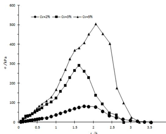
**Figure 3.** Stress-strain curves of artificially sand in 7 days.
