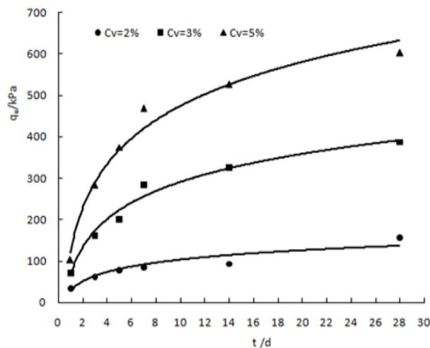
**Figure 7.** Relationships between unconfined compressive strength ( $q_u$ ) and curing time ( $t$ ) of artificially cemented sand.
