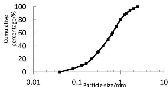
**Figure 1.** Standard sand sample particle grading curve.
