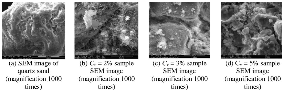
**Figure 4.** SEM photos of cement sample in 7 days.
