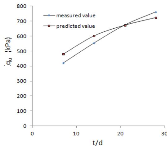
**Figure 8.** Comparison of measured value and predicted value of unconfined compressive strength of cemented sand with ratio of 8%.
