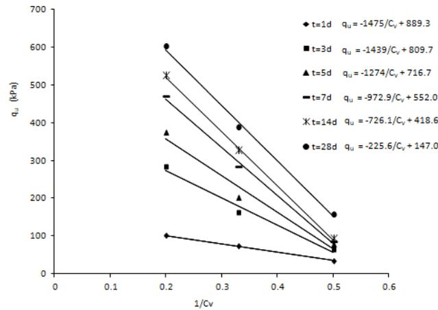
**Figure 5.** Relationships between unconfined compressive strength ( $q_u$ ) and clinker cement ratio ( $C_v$ ) of artificially cemented sand.
