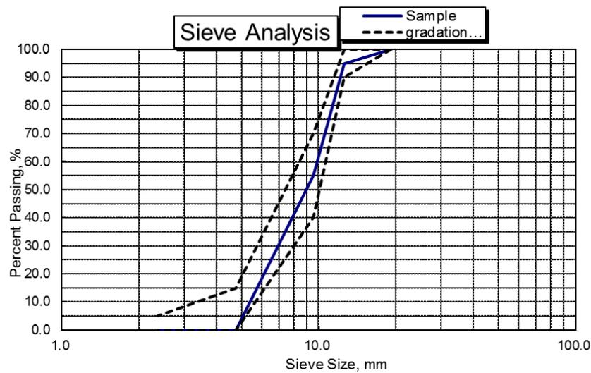
**Figure 1.** Aggregate gradation used in this study [18]
