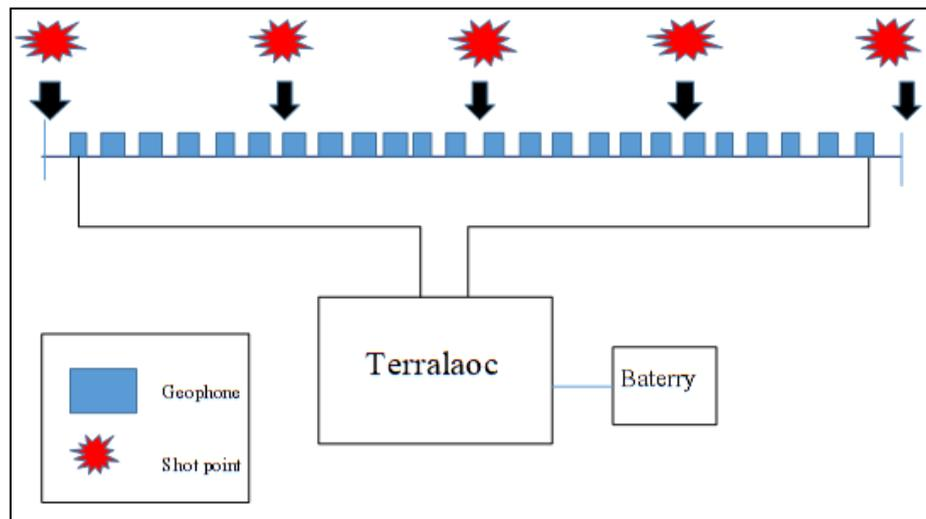
**Figure 2.** The setting of the seismic survey lines and location of the shot points
