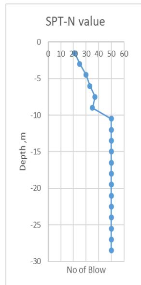
**Figure 3.** SPT-N value of the site from borehole
