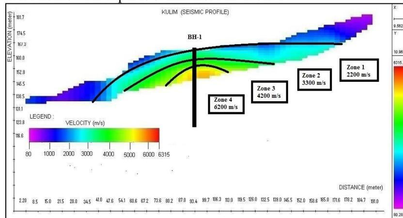
**Figure 5.** Seismic profile divided into four different zones
