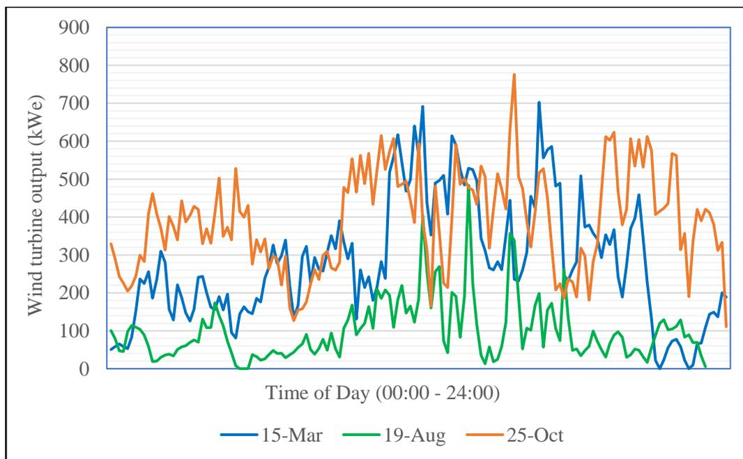
**Figure 1.** The daily output of a wind turbine in Ireland.
