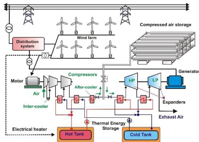
**Figure 3.** Simplified diagram of distributed compressed air energy storage.
