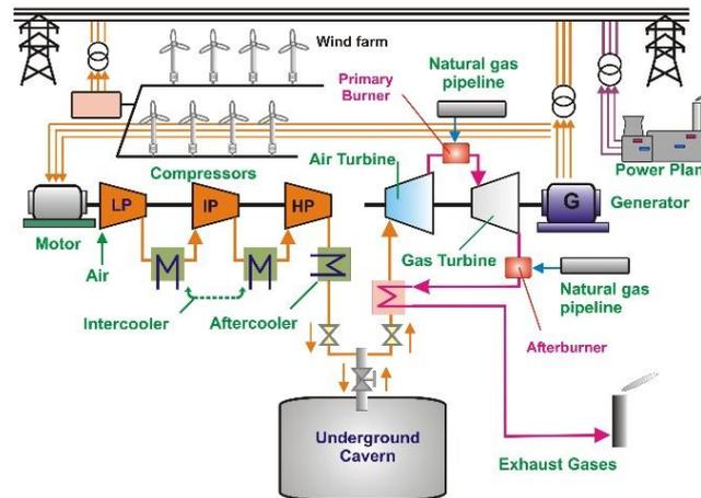
**Figure 2.** Simplified diagram of grid scale compressed air energy storage.
