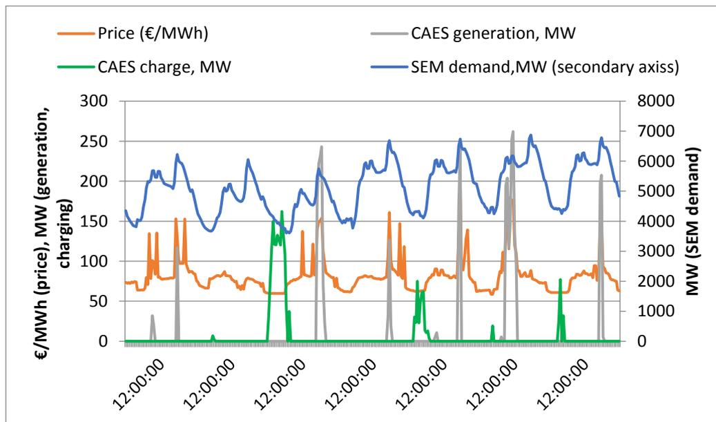
**Figure 4.** Operational profile for the CAES system in the SEM.
