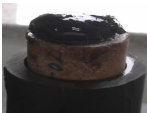
Figure 4. The core sample plugged by water soluble temporary plugging agents.
