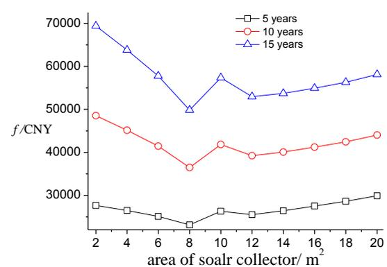
**Figure 6.** Total cost of the system with different operating years. (Volume of buffer is 1200 L, tilt angle of collectors is 45 degree).
