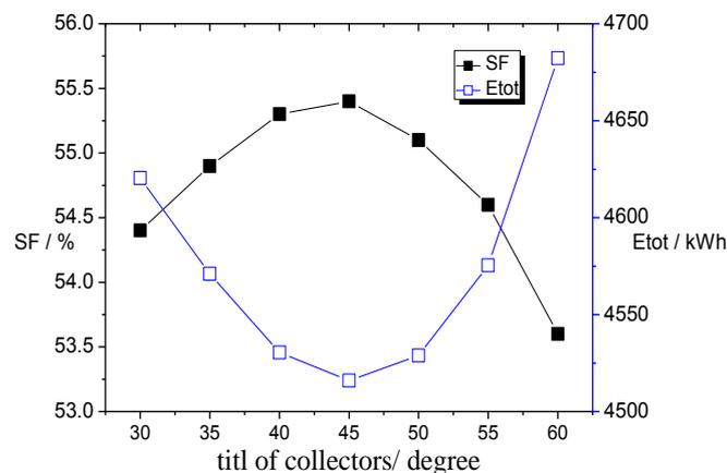
**Figure 3.** Relationship between tilt angle of collectors and  $SF$ ,  $E_{tot}$ . (Area of solar collectors is 10 m<sup>2</sup>, volume of buffer is 800 L).
