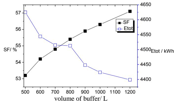
**Figure 4.** Relationship between volume of buffer and  $SF$ ,  $E_{tot}$ . (Area of solar collector is 10 m<sup>2</sup>, tilt angle of collectors is 45 degree).
