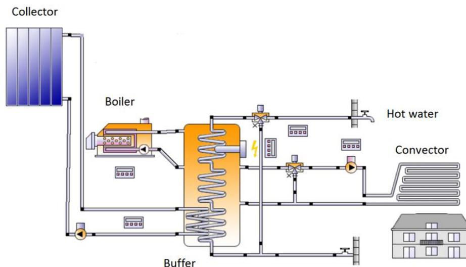
**Figure 1.** A solar thermal system designed using Polysun.
