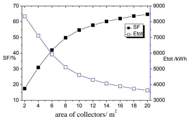
**Figure 5.** Relationship between area of collectors and  $SF$ ,  $E_{tot}$ . (Volume of buffer is 1200 L, tilt angle of collectors is 45 degree).
