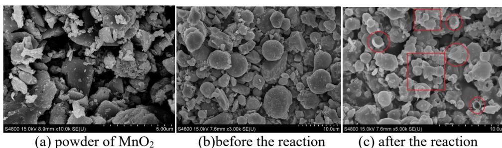
(a) powder of  $\text{MnO}_2$  (b) before the reaction (c) after the reaction
