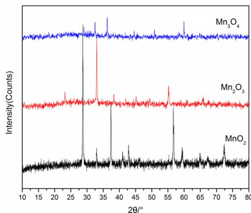
Fig.2 XRD spectrum of MnO<sub>2</sub> and its thermal decomposition products
