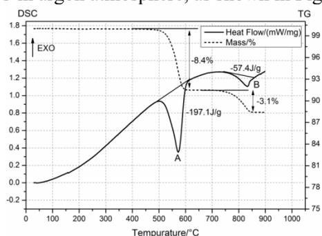
Fig.1 The TG-DSC curve of MnO<sub>2</sub> powder
