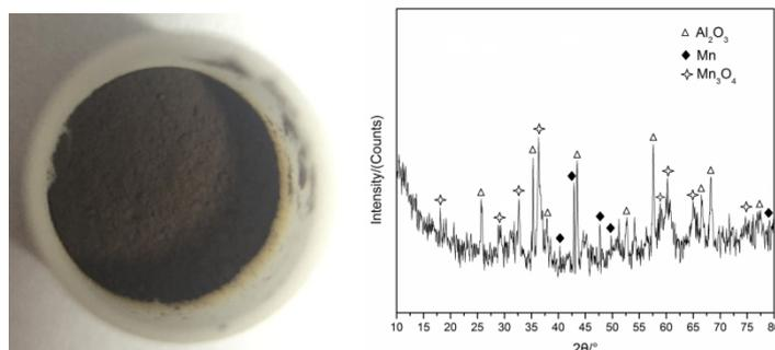
Fig.4 products after reaction Fig.5 XRD pattern of the reaction products
