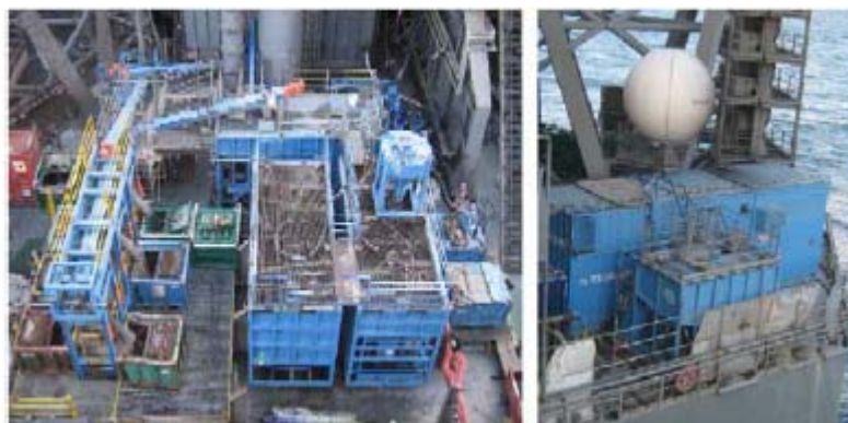
(b) TCC applied in offshore oil field
