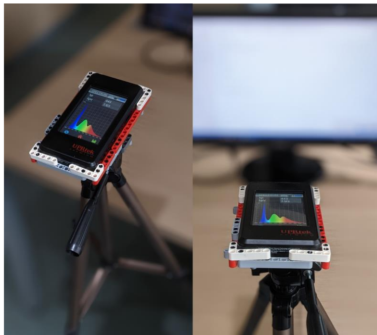
Figure 2. Spectrometer mounted on the tripod making measurements on a monitor.
