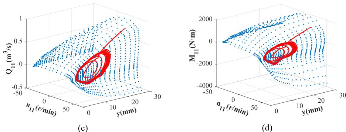
**Figure 9.** Discharge and torque operating trajectory (reduce active power command): (a) discharge: speed command -8%; (b) torque: speed command -8%; (c) discharge: speed command +8%; (d) torque: speed command +8%.
