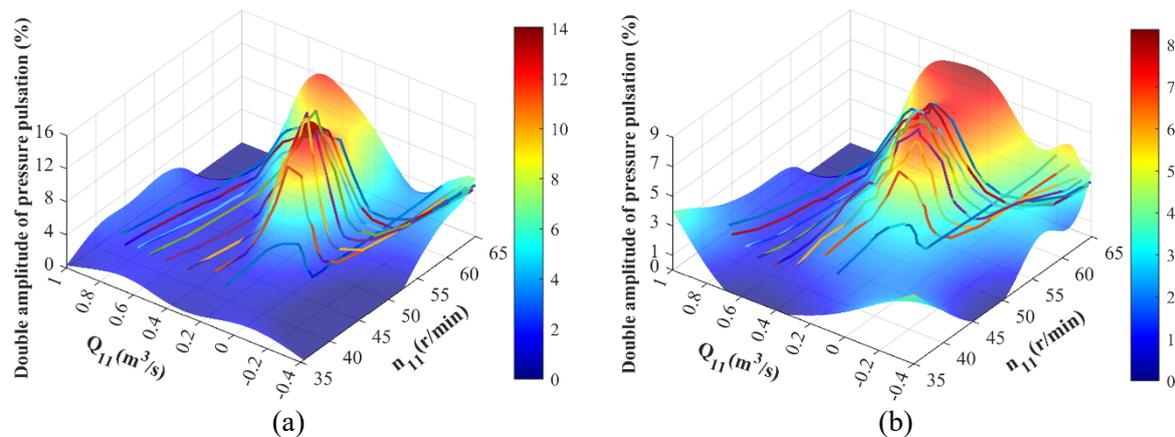
**Figure 2.** The three-dimensional surface of pressure pulsation: (a) volute inlet; (b) draft tube.
