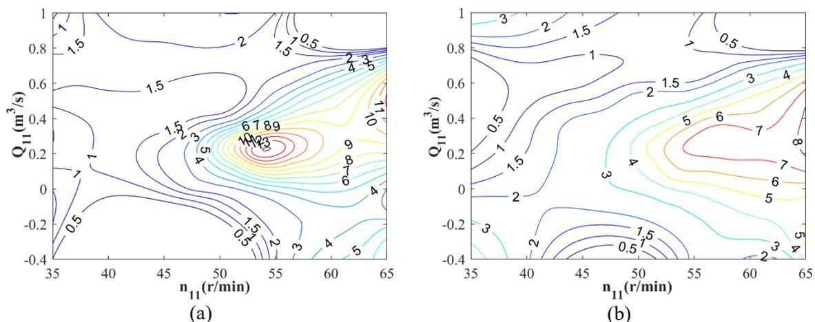
**Figure 1.** The double-amplitude contour of pressure pulsation: (a) volute inlet; (b) draft tube.
