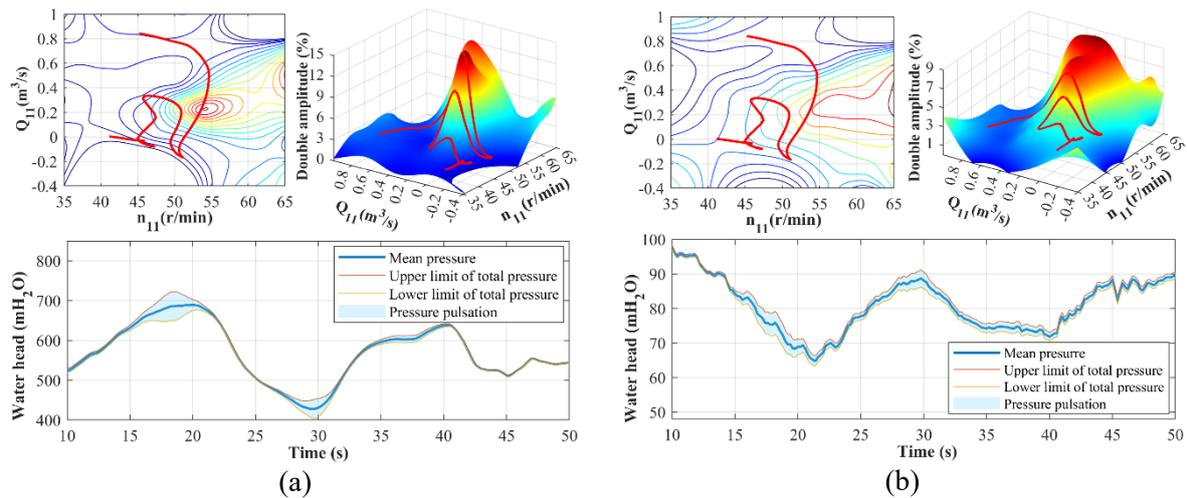
**Figure 3.** Operating trajectory and predicted total pressure: (a) volute inlet; (b) draft tube.
