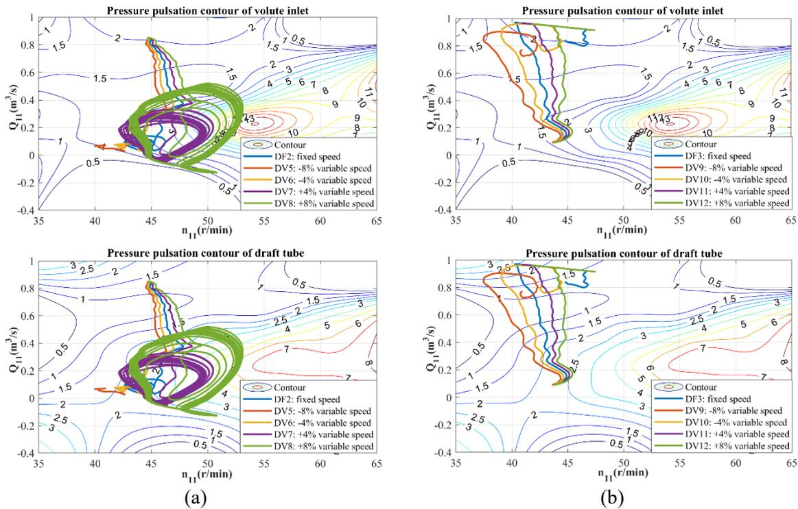
**Figure 8.** Evolution diagram of operating trajectory (changing speed command): active power command - (a) reduce; (b) increase.
