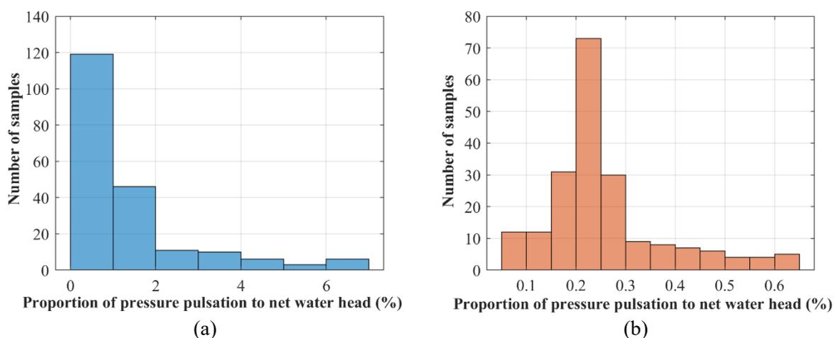
**Figure 4.** Histogram of the proportion of pressure pulsation: (a) volute inlet; (b) draft tube.
