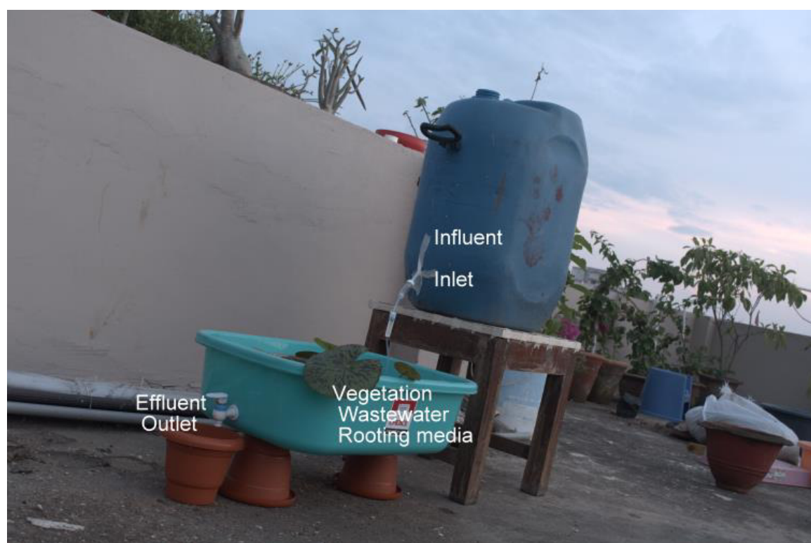
Figure 3. Vertical Type Constructed Wetland
