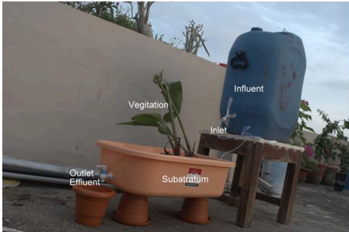
Figure 4. Horizontal Flow Constructed Wetland (HFCWs)
