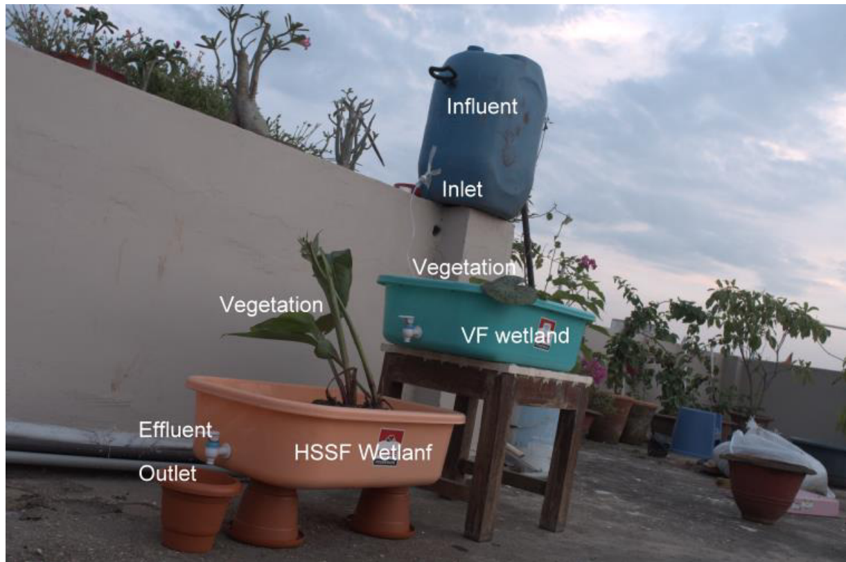
Figure 5. Hybrid Constructed Wetland (HCWs)
