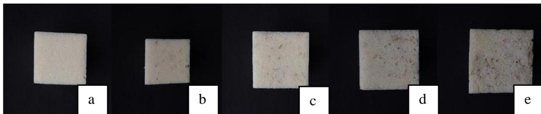
**Figure 13.** Cross section of RPUFC with density  $60 \text{ kg/m}^3$ : (a) 0% bagasse; (b) 2.5% bagasse; (c) 5% bagasse; (d) 7.5% bagasse; and (e) 10% bagasse.
