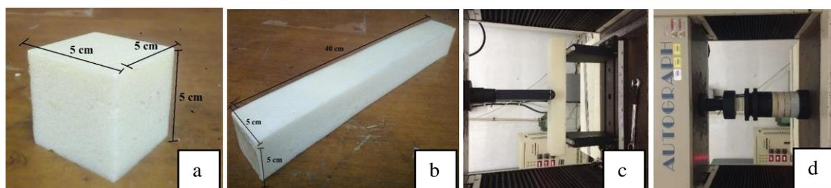
**Figure 3.** Foam size and testing process: (a) foam 5 × 5 × 5 cm, (b) foam 40 × 5 × 5 cm, (c) FS test, and (d) CS test.
