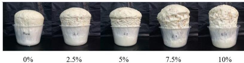
**Figure 4.** RPUFC free rise foaming conditions by the effect of adding SB particles.
