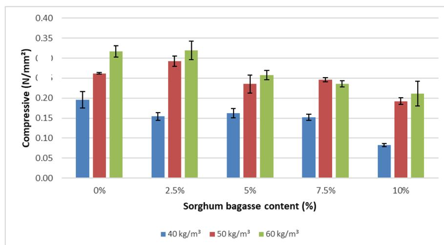
**Figure 10.** Compressive strength values of RPUFC.
