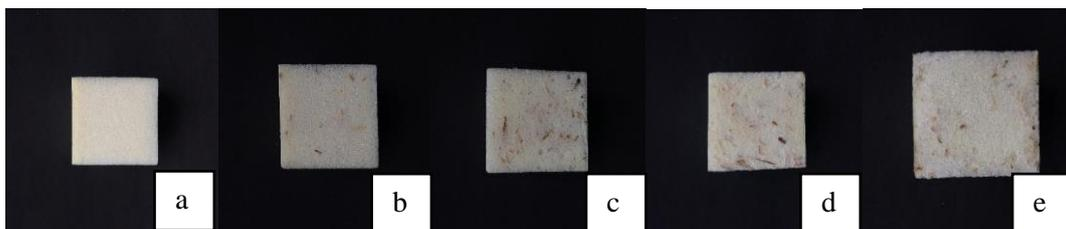
**Figure 12.** Cross section of RPUFC with density  $50 \text{ kg/m}^3$ : (a) 0% bagasse; (b) 2.5% bagasse; (c) 5% bagasse; (d) 7.5% bagasse; and (e) 10% bagasse.
