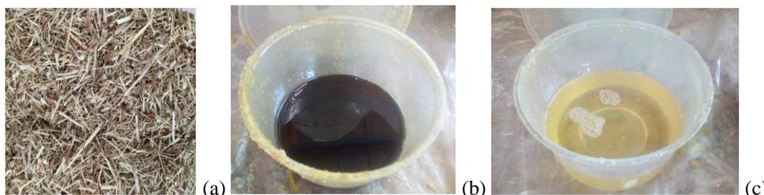
**Figure 1.** The used materials for RPUFC: (a) sorghum bagasse particle, (b) isocyanate, (c) polyol.
