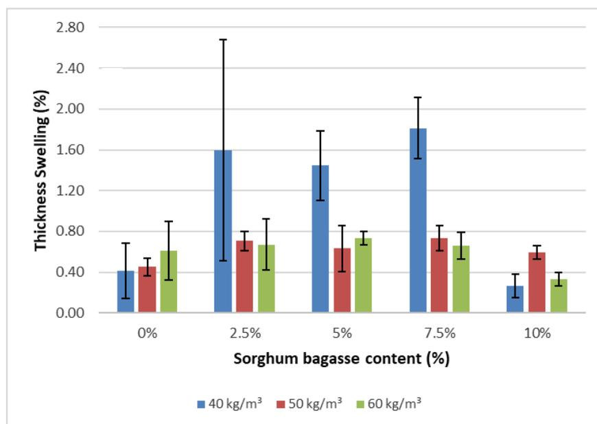
**Figure 7.** Thickness swelling of RPUFC.
