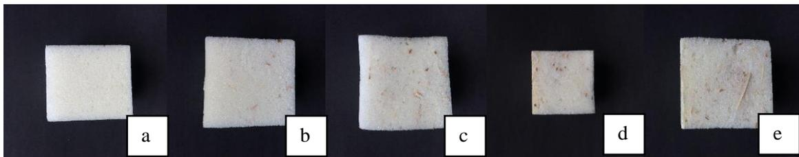
**Figure 11.** Cross section of RPUFC with density  $40 \text{ kg/m}^3$ : (a) 0% bagasse; (b) 2.5% bagasse; (c) 5% bagasse; (d) 7.5% bagasse; and (e) 10% bagasse.
