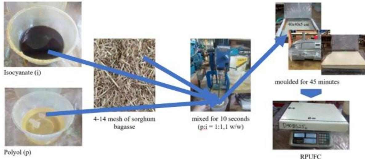
**Figure 2.** Manufacture of the RPUFC.
