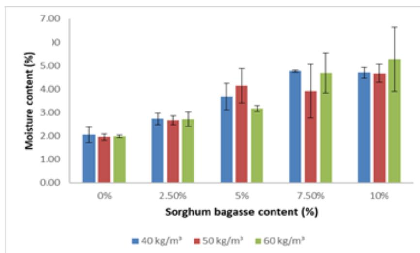
**Figure 5.** The moisture content of RPUFC.
