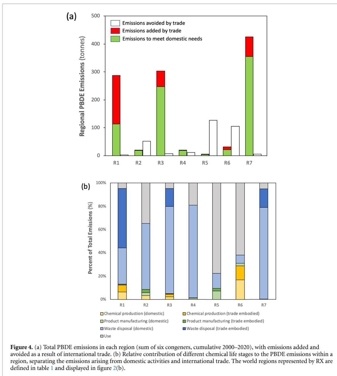
emissions added through the production of PBDEs destined for export are much smaller than the emissions avoided through the export of PBDE containing waste.
