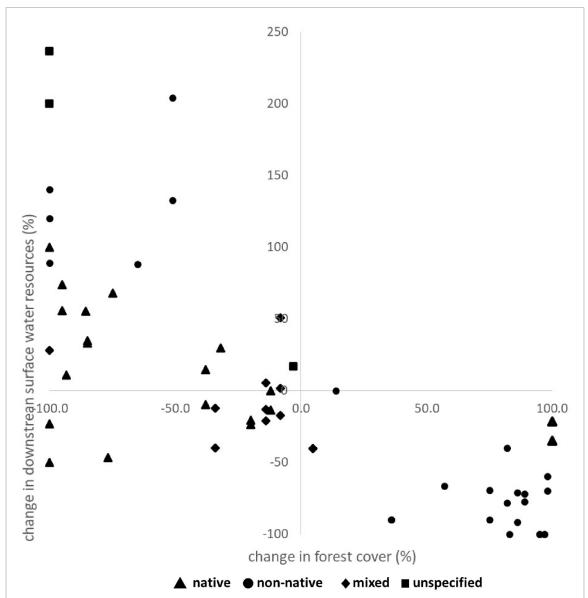
**Figure 2.** Relationship between change in forest cover (% of catchment area) and change in downstream surface water resource quantity (%). The vertical axis is truncated at 250% to aid visualisation of lower values, which excludes the four most extreme increases in resource quantity due to deforestation (maximum 3450%).
