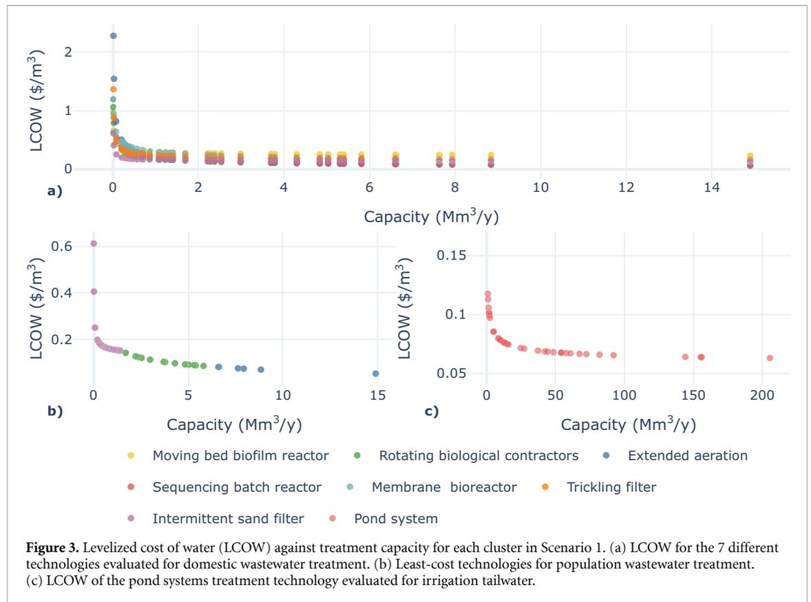
**Figure 3.** Levelized cost of water (LCOW) against treatment capacity for each cluster in Scenario 1. (a) LCOW for the 7 different technologies evaluated for domestic wastewater treatment. (b) Least-cost technologies for population wastewater treatment. (c) LCOW of the pond systems treatment technology evaluated for irrigation tailwater.
