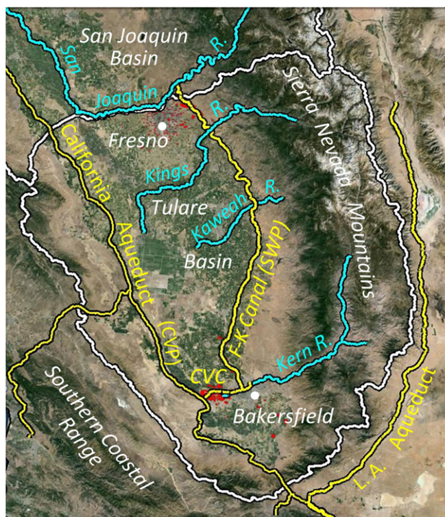
Figure 1. Infrastructure to support conjunctive use and managed aquifer recharge (MAR) in the southern California Central Valley. The primary basins are the San Joaquin and Tulare basins. Infrastructure to import water from the north includes the Friant–Kern (F–K) Canal (Central Valley Project, CVP), California Aqueduct (State Water Project, SWP), and the Cross Valley Canal (CVC) linking CVP and SWP ( www.water.ca.gov/swp/cvp.cfm/ ). The MAR systems (shown in red) are located near the cities of Bakersfield (Kern County) and Fresno (Fresno County).
