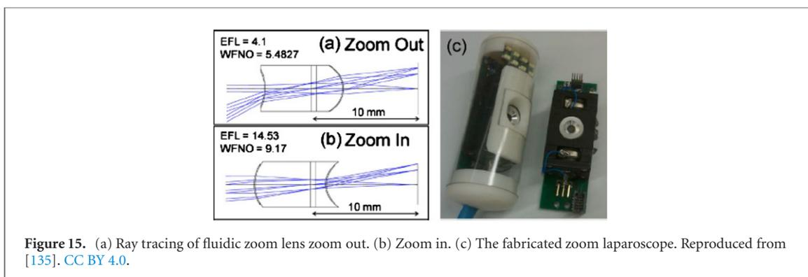
**Figure 15.** (a) Ray tracing of fluidic zoom lens zoom out. (b) Zoom in. (c) The fabricated zoom laparoscope. Reproduced from [135]. CC BY 4.0.
