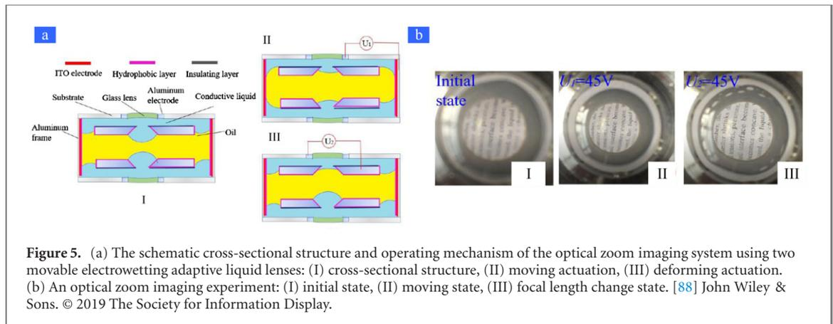
**Figure 5.** (a) The schematic cross-sectional structure and operating mechanism of the optical zoom imaging system using two movable electrowetting adaptive liquid lenses: (I) cross-sectional structure, (II) moving actuation, (III) deforming actuation. (b) An optical zoom imaging experiment: (I) initial state, (II) moving state, (III) focal length change state. [88] John Wiley & Sons. © 2019 The Society for Information Display.
