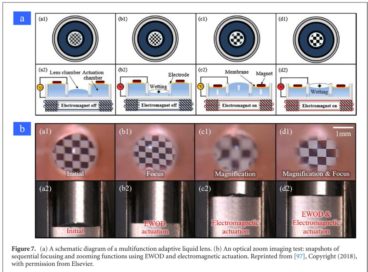
**Figure 7.** (a) A schematic diagram of a multifunction adaptive liquid lens. (b) An optical zoom imaging test: snapshots of sequential focusing and zooming functions using EWOD and electromagnetic actuation. Reprinted from [97], Copyright (2018), with permission from Elsevier.
