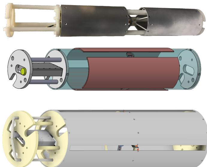
**Figure 14.** Photo of a Vpol prototype (top) and technical drawings of options for the Hpol antennas (trislots, middle, quadslots, bottom). The Vpol and trislots are the first iterations of the deep antennas for RNO-G, while the quadslot is being considered for use in conjunction with larger diameter boreholes.
