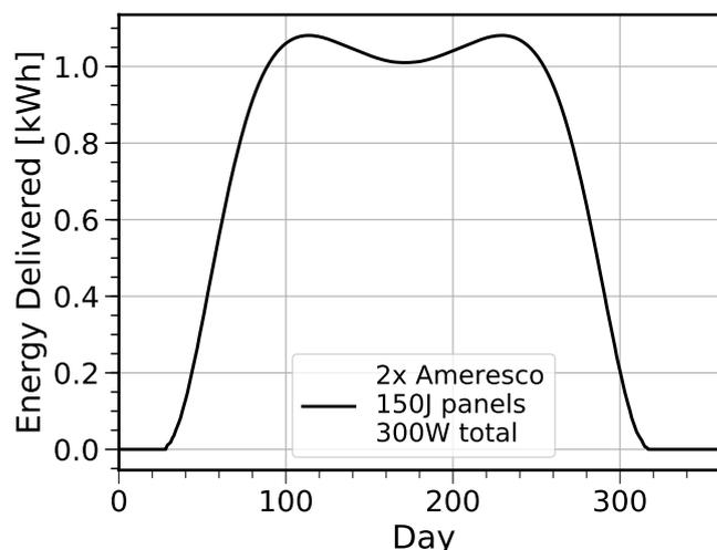
**Figure 20.** Predicted daily energy delivered by a 300 W photo-voltaic (PV) array to an RNO-G station at Summit Station. The PV array comprises two Ameresco 150J rugged panels mounted vertically and facing south. The total PV area is  $2\text{ m}^2$ .
