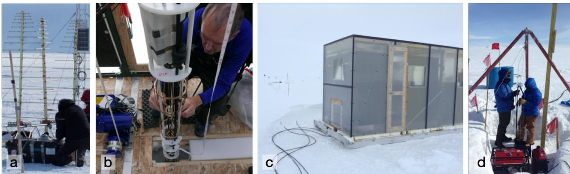
**Figure 23.** RNO-G installation plans are based on prior deployments of (a) surface stations at ARIANNA and (b) strings of antennas deployed in boreholes for ARA, both in compact phased arrays and reconstruction strings. A deployment shed for the drill and installation will be built on skis based on prior work done for ARA (c). Site studies conducted at Summit Station in Greenland also informed the installation plans (d).
