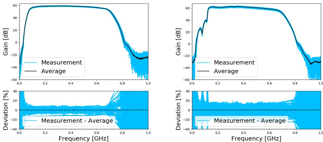
**Figure 17.** Gain of the RNO-G amplifiers. Left: 12 SURFACE amplifiers. Right: combination of 23 IGLU and DRAB amplifiers, including a 50 m optical fiber cable. All amplifiers are revision v1 hardware.
