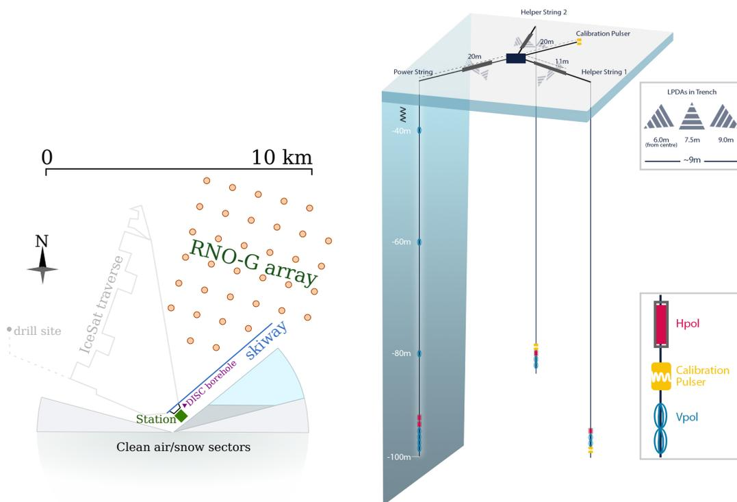
**Figure 7.** Left: map of the planned RNO-G array at Summit Station; grid spacing is approximately 1 km. Right: a single RNO-G station consists of three strings of antennas (Hpol and Vpol) plus surface antennas (LPDAs), as well as three calibration pulsers located both deep in the ice and also at the surface. The string containing the phased array trigger is designated as the *power string*, while the two additional strings are designated as *support strings*.
