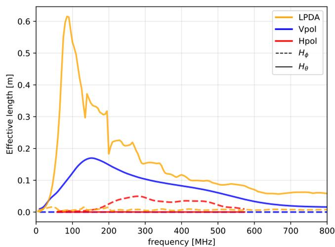
**Figure 15.** Antenna effective length magnitude for the LPDA, Vpol and Hpol (tri-slot) in the direction of maximum gain  $H_\theta$  (V-pol and LPDA) or  $H_\phi$  (H-pol). Results of detailed antenna simulations of the v1 iterations as shown in figure 14.
