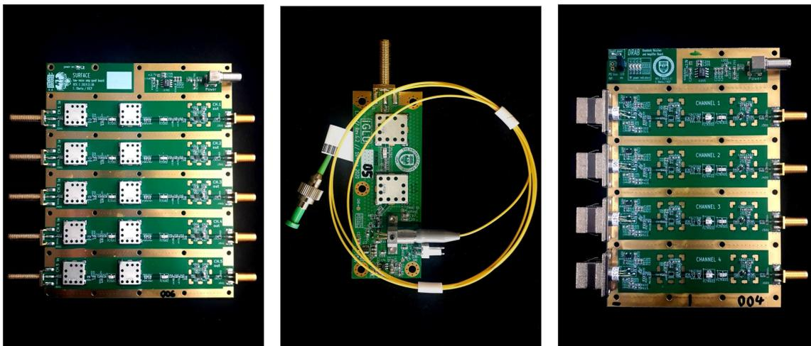
**Figure 16.** Amplifiers as designed for RNO-G. Left: SURFACE amplifiers for the signals coming from the LPDAs via coaxial cable. Middle: an IGLU board (In-ice Gain with Low-power Unit) used to convert signals from antennas deep in the ice to analog RF signals and then feed them into the indicated fiber. Right: DRAB board (Down-hole Receiver and Amplifier Board) located within the station housing. All amplifiers are shown without their environmental enclosures.
