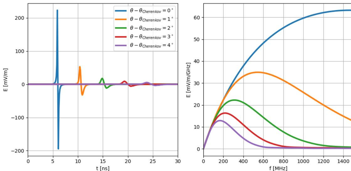
**Figure 4.** Electric-field waveforms (left) and spectra (right) of the radio signal emitted at different viewing angles relative to the Cherenkov angle, for a hadronic shower with energy deposition of 1 EeV. For enhanced readability, the waveforms have been offset in time. No propagation or detector effects have been included.
