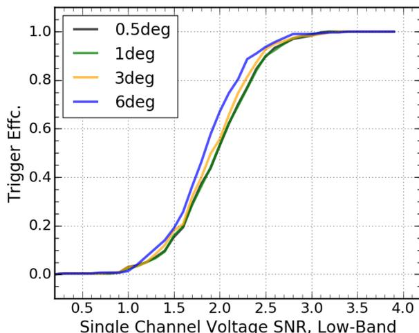
**Figure 18.** End-to-end simulation of the 4-antenna phased array trigger design for RNO-G. The simulated trigger efficiency for a number of neutrino signals at different off-cone viewing angles in the trigger bandwidth of 80 MHz–250 MHz.
