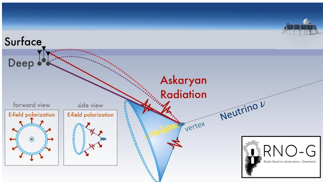
**Figure 5.** Schematic of the detection of the radio emission following a neutrino interaction (not to scale). The emission is strongest at the Cherenkov angle (blue cone) and can follow straight and bent trajectories to the receiving station depending on the profile of the index of refraction of the ice. The signal is usually detected at large distances and is strongly polarized as illustrated in the insets.
