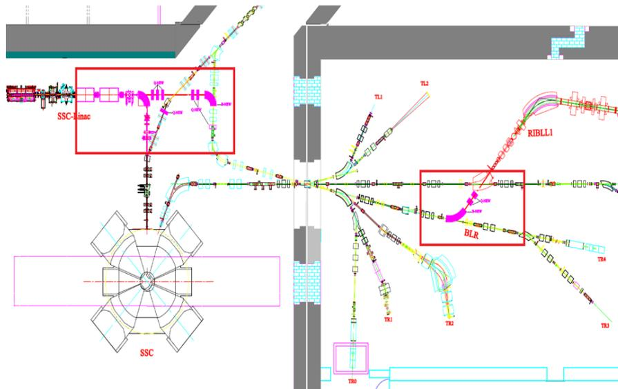
**Figure 9.** By-pass beam lines (in red box) will be constructed to improve the operation efficiency.
