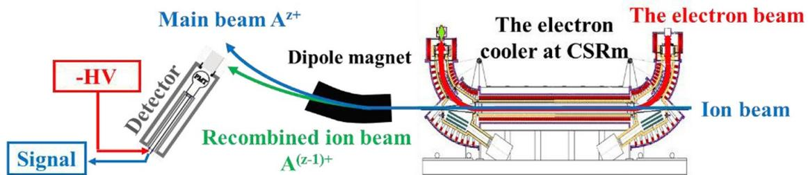
Figure 6. Sketch of the DR experimental setup at HIRFL.
