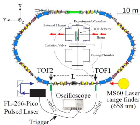
**Figure 5.** Schematic view of the storage ring CSRe and its double TOF detectors.
