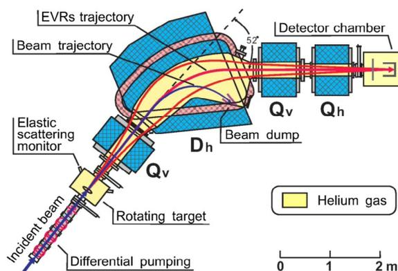
**Figure 4.** A schematic view of the gas-filled recoil separator SHANS.
