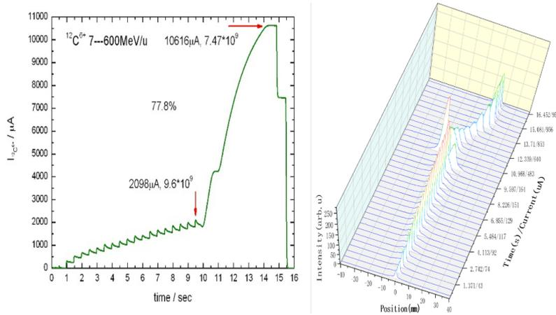
Figure 8. Beam current and horizontal profile measured in CSRm during one operation cycle.
