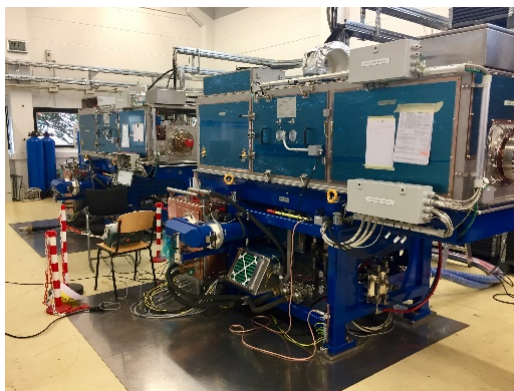
Figure 10. Series production of SIS100 acceleration cavities and factory acceptance tests.
