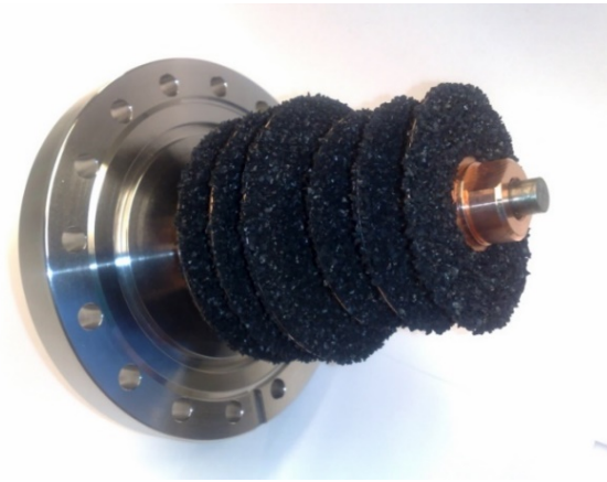
Figure 3. Cryosorption pump using charcoal for H pumping.
