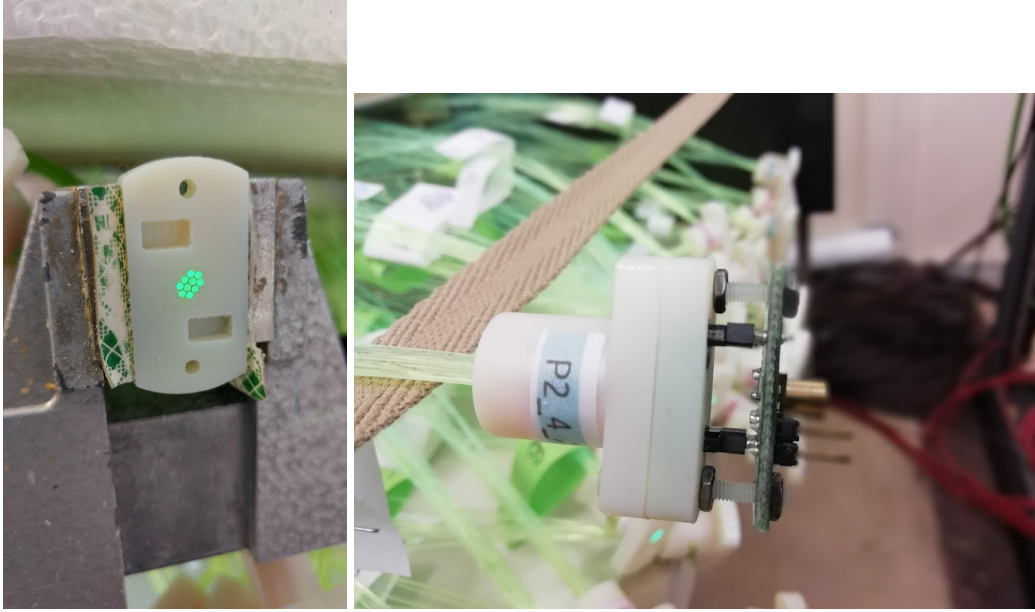
Figure 7. Left: fiber connector close up. Right: detail of the SiPM's connector.
