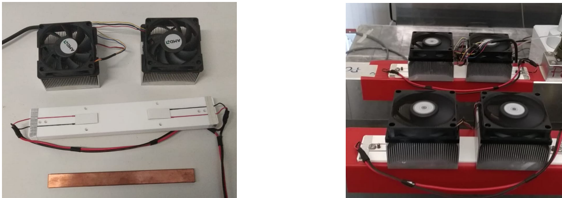
Figure 4. Temperature control system, before and after mounting on the detectors.
