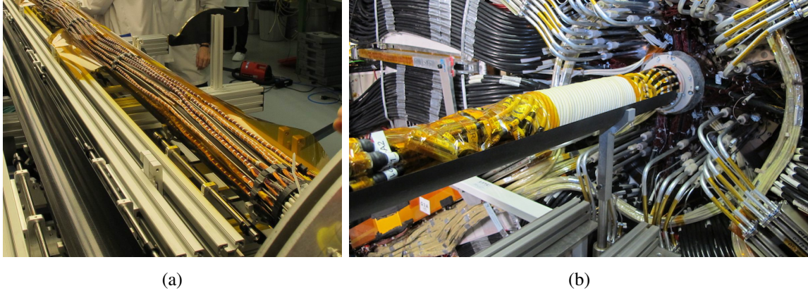
Figure 58. (a) Type 1 services integrated on the Inner Positioning Tube (IPT) and Z-stopper locked into the service rings. (b) Spiral wrapped Type 1 cables that take up the excess length of the IBL envelope and limit the radial envelope with respect the Inner Support Tube (IST) for the insertion.
