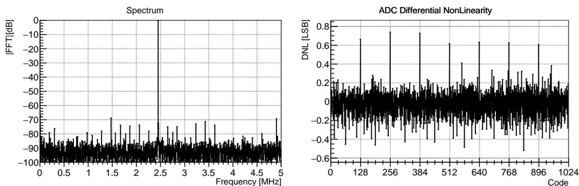
**Figure 4.** Measured performance of SAMPA prototype\_2 ADC at 10 MSps: spectrum in presence of 2.45 MHz sine wave (left), Differential Non-Linearity (DNL) in the same conditions (right).
