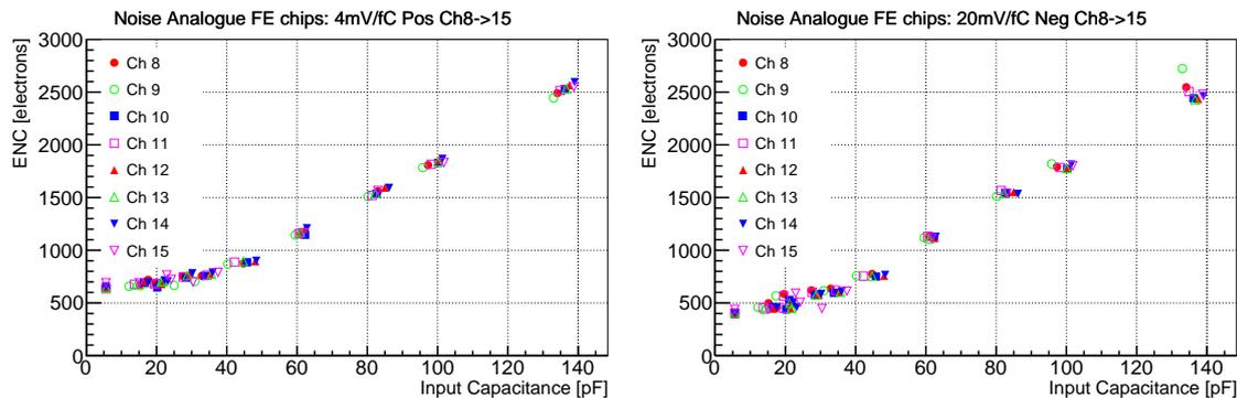
**Figure 3.** Noise, expressed in ENC, for 4 mV/fC (left) and 20mV/fC (right) configurations in various channels of one of the analogue front-end test-chip sample. ENC was calculated using nominal gain.
