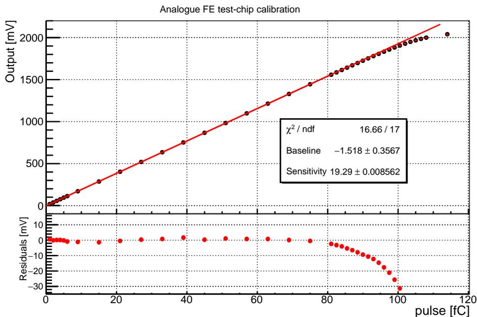
**Figure 2.** Analogue front-end test-chip: a calibration curve for the configuration 20 mV/fC.
