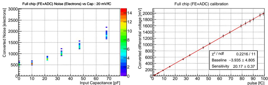
**Figure 5.** An example of full chip results, configuration 20 mV/fC. Left, noise, expressed in ENC (assuming nominal gain), colors represent number of channels in a noise bin. Right, a calibration curve. In both cases ADC values were converted using the nominal 2.15 mV/LSB factor.
