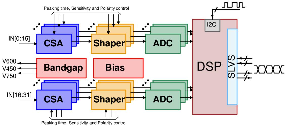
**Figure 1.** Sampa block diagram.
